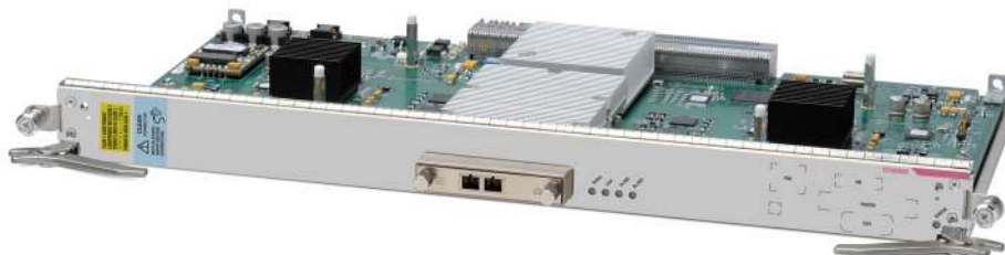
Figure 1. Cisco CRS-3 1-Port 100 Gigabit Ethernet Interface Module
