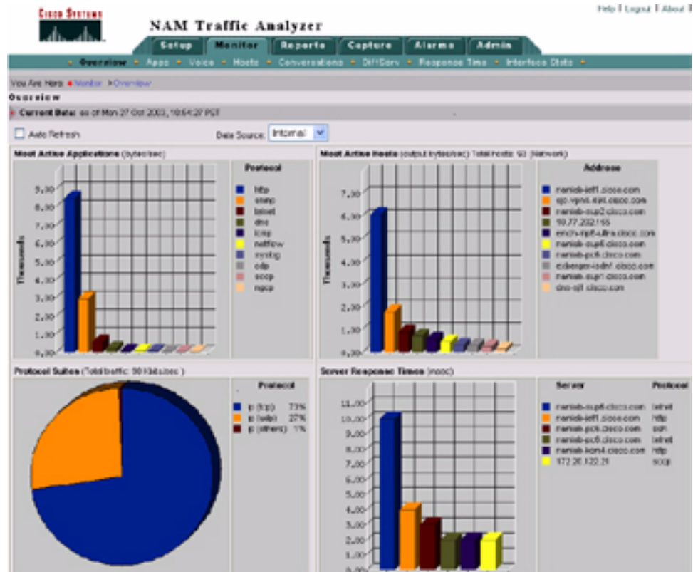
Figure 2 Web-Based Traffic Monitoring for the LAN and WAN with the Embedded NAM Traffic Analyzer
